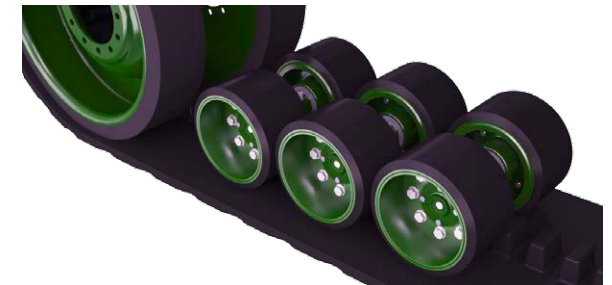
Wide wheels with wide tracks reduces ground pressures and prolongs track life
