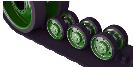
Narrow wheels on wide tracks leads to shorter track life and higher ground pressures
